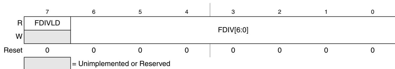
Figure 23-5. Flash Clock Divider Register (FCLKDIV)
