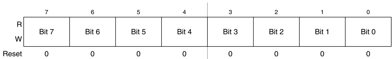
Figure 21-23. Timer Input Capture/Output Compare Register x Low (TCxL)
